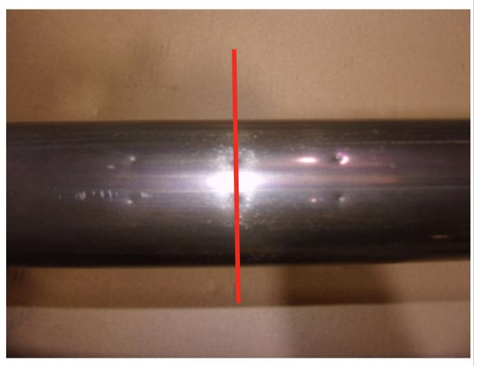
To make it easier to cut the exhaust we reccomend remoiving it from the car. Find the 3 pairs of indents and use the middle pair to mark out the cutting line. Cut along the line and de-bur the edges. Re-fit the original GPF and fit the Scorpion GPF-back following the line diagram above.
